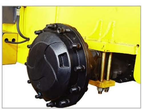
Hydraulic heavy duty vibratory rollers are suitable for compaction of non-cohesive materials such as gravel, crushed stone, sand-macadam mixture, sandy soil and rock filling etc. on base course, sub-base and embankment fill construction, which are ideal equipment for high-class highway, railway, airport, harbors, dams and large-scale industrial ground.
